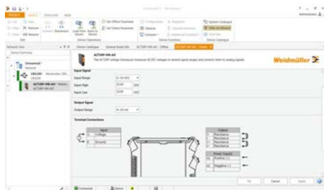
screenshot of configuration with FDT2 / DTM software
