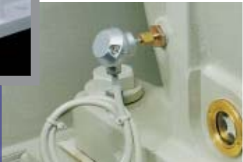
Pt-100 bearing temperature detector and oil sight-glass
