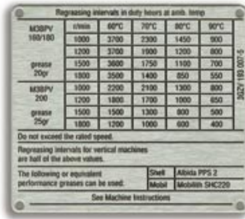
Lubrication plate for frame sizes 160-200.
