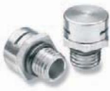
The DAE pressure-compensation element provides good ventilation for the enclosure and prevents moisture build-up. At the same time it maintains the high IP69k protection level. The membrane repels water and oil.
