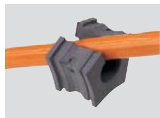
2. Press the grommet with the cable into the open cable gland. The flat sides of the grommet must face upwards when fitting the KVT 63/4!
