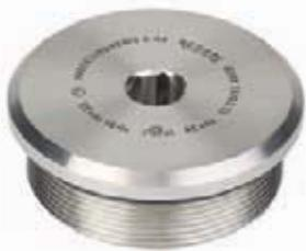
Dome head sealing plug with accessible hexagon recess. It is used to seal unused threaded holes so that cable glands can be connected in the future. Available in brass and stainless steel. Approved for use with the pressure-resistant Ex d encapsulation and increased safety Ex e.
