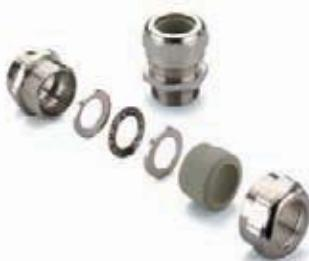
Brass cable gland for shielding against interference frequencies with a screening attenuation of up to 100 dB. Contact with cable shield by means of spring washer.
