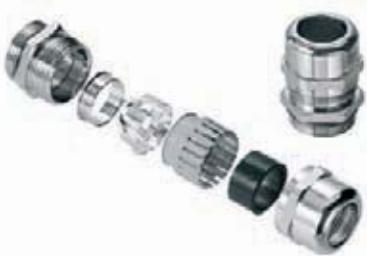
Brass cable gland for shielding against interference frequencies with a screening attenuation of up to 90 dB. Conical metal cage ensures multiple contacts with the cable shielding.
