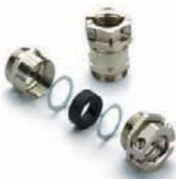
Brass cable glands with external, centrally positioned strain relief provided by the clamping jaws.
