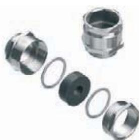
Brass cable gland with concentric O-rings for standard industrial applications. The sealed insert used here contains several removable or dividable inlets. This allows to connect cables of a wide diameter range (from 4 mm to 41 mm) with only one sealed insert.
