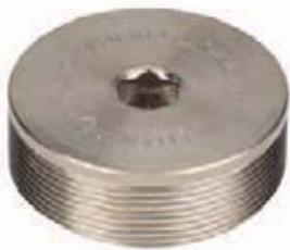
Sealing plug with accessible hexagon recess. It is used to seal unused threaded holes so that cable glands can be connected in the future. Approved for use with the pressure-resistant Ex d encapsulation.
